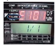
Note: if no alarms are stored in controller bottom display will read 0/0. Alarm codes are displayed on top display and alarm date and time are displayed in bottom display.
